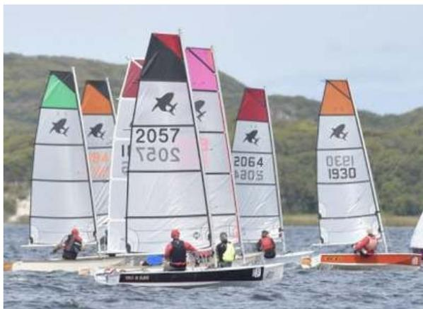
The December issue of *The Main Sheet* included a photo of the new phenomenon that is the square-top sail for the Sabre dinghy. Known as the Shark sail, it is a made of Mylar, has full-length battens and is cut with the head square to the mast.
